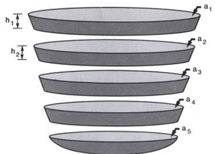
Figure 9. During a bathymetric survey of a lake, depths are measured along transect lines. When the map is constructed, points of equal depth are connected by contour lines.
