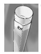
2 Add one pH tablet to the sample in the tube.
