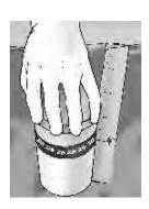
Remove the sampling container from the water, read the temperature and record it in degrees Celsius.
