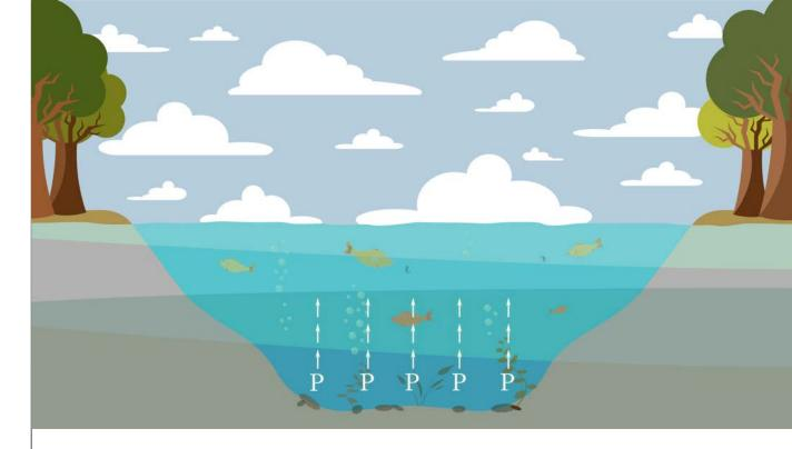
Phosphorus released from the bottom sediments triggers algae growth
